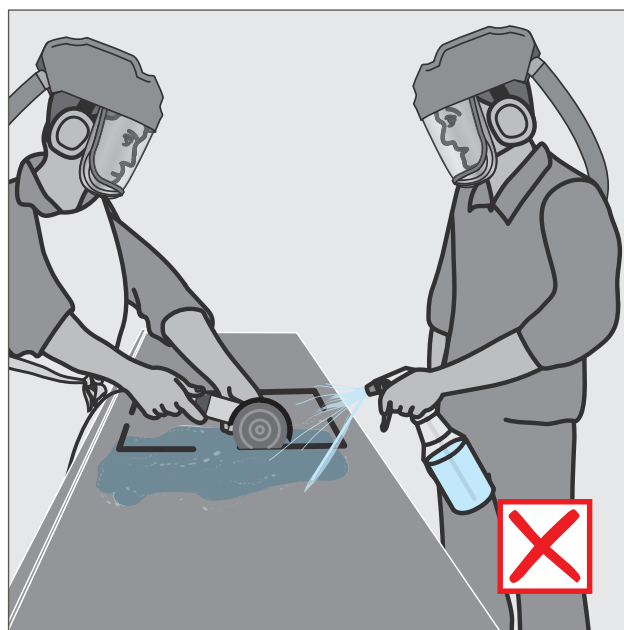
Figure 6(d): Inappropriate water suppression: use of spray bottle
